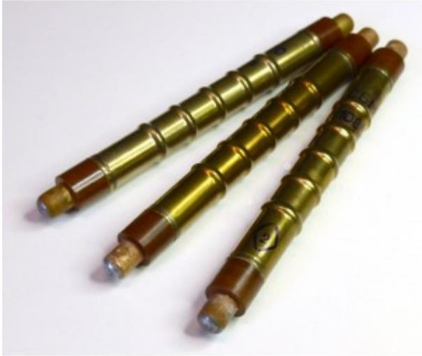
Among the russian tubes, this one is the favourite of ours to measure gamma and beta radiations, because it's the most sensitive to this kind of radiation in its price class. To further enhance the already good sensitivity, you may just parallel two devices and you get double sensitivity without any special circuit. Tubes come from russian warehouses: they're used, but checked for good operational status.
